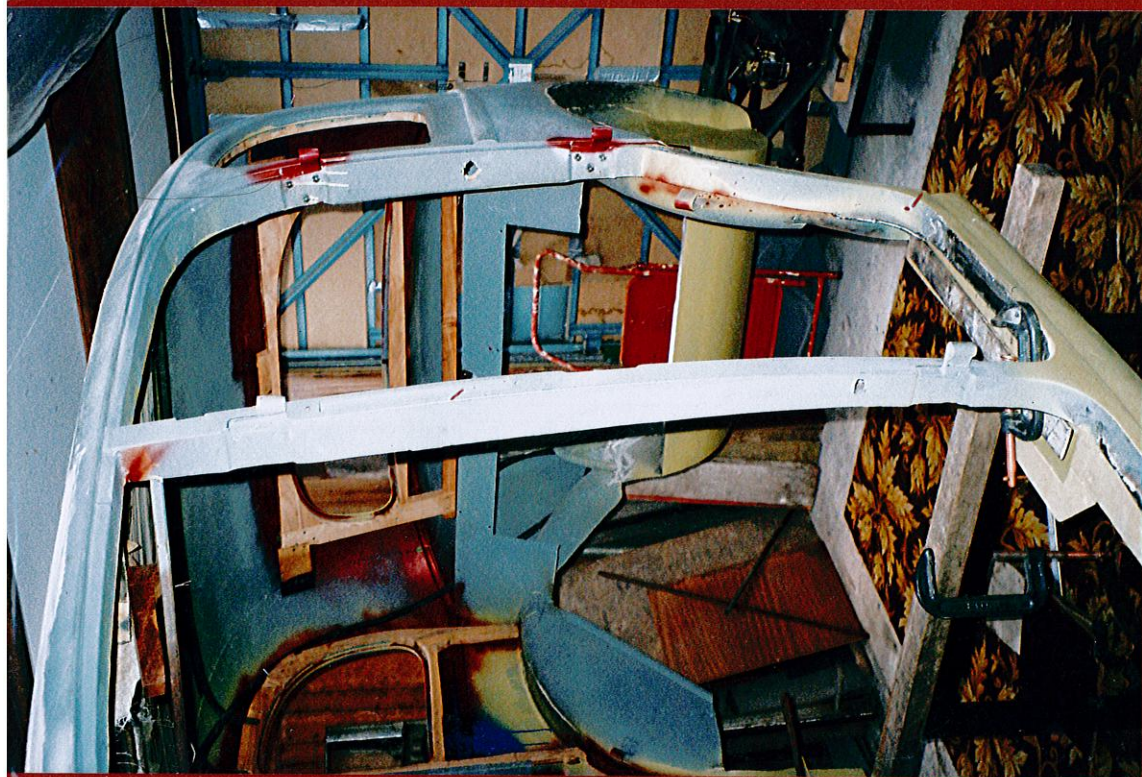
Memo Ash Frame Memo being fitted
