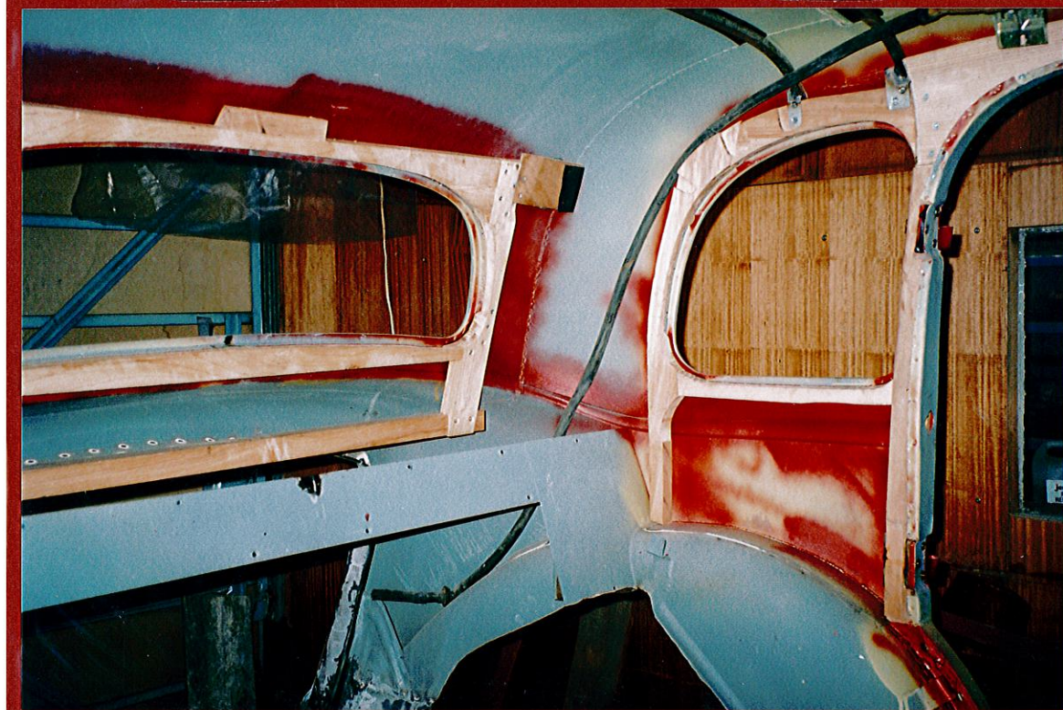
Memo Ash Frame Memo being fitted
